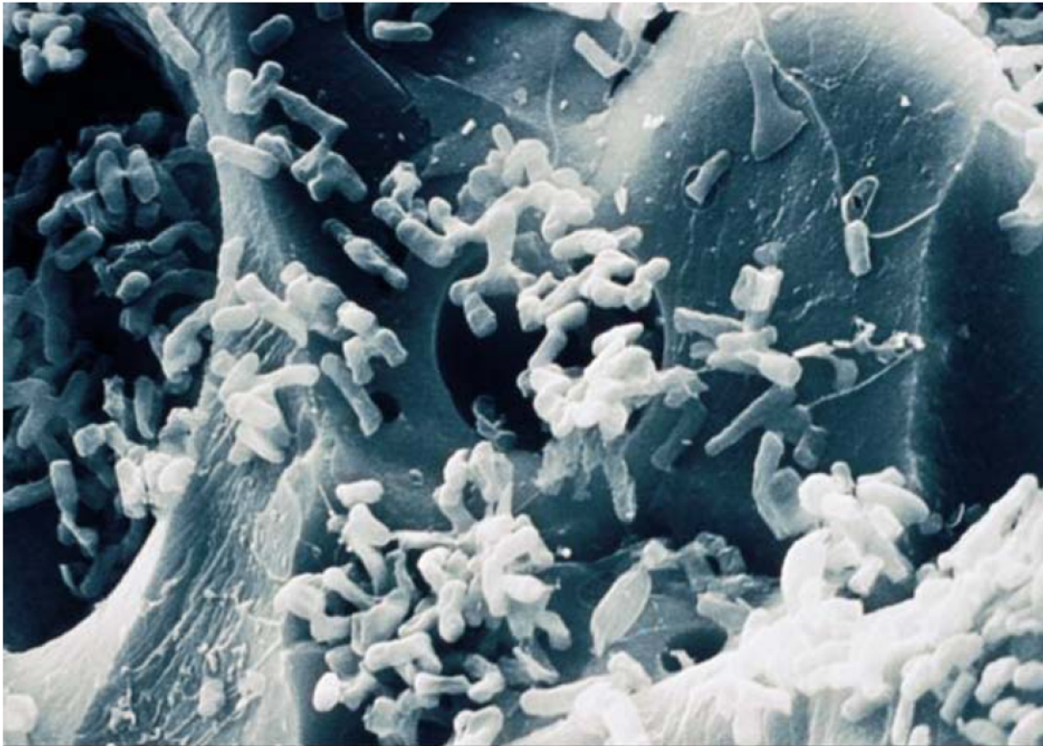
Picture2: Electron microscope photograph of bacteria cells attached to expanded clay (Filtralite).
