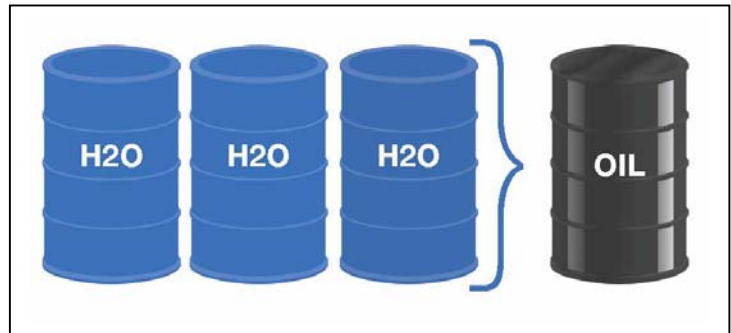
Producing oil from the tar sands takes on average three barrels of freshwater to make one barrel of oil
